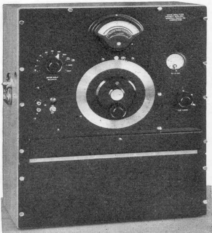
FIGURE 1. Above the frequency-control dial of the wave analyzer is the voltmeter shown in FIGURE 2. At the left is the meter multiplier
